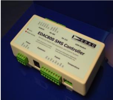
The EDAC 800 SMS Controller has four inputs and four outputs that can be independently configured.
